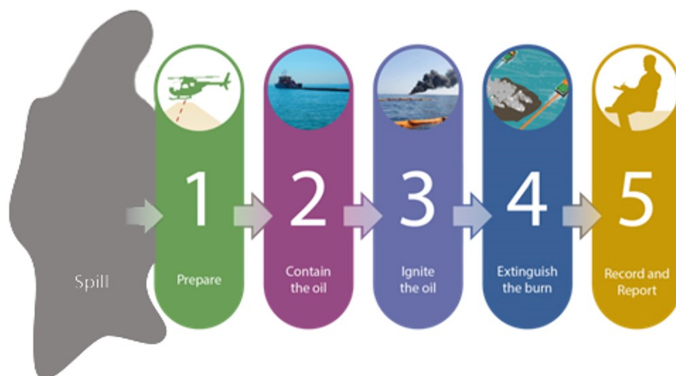
Figure 15: In Situ Burning Key Steps
